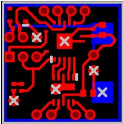
Some of the goofy routing is due to the large minimum via size of .024" that the manufacturer was limited to.
